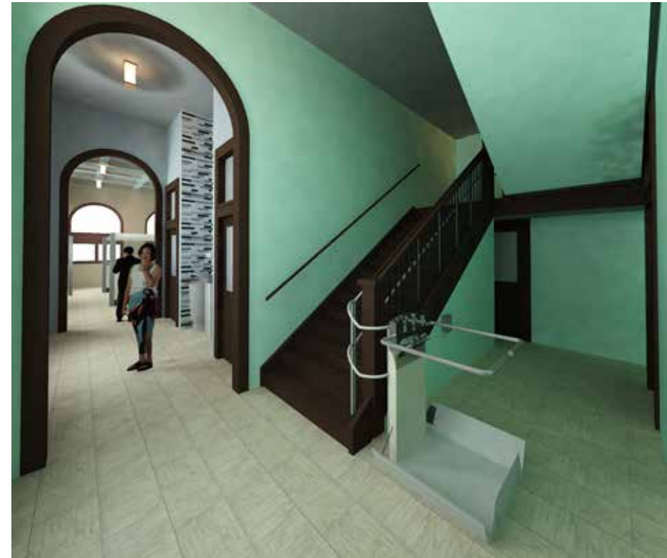
Existing Lobby Stair and New ADA Lift
